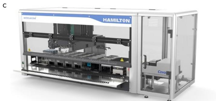
**Figure 2.** Automated library preparation on the Hamilton STARplus with (A) 96-well pipetting heads, (B) on-deck thermocycler and (C) Covaris R230 Focused-ultrasonicator.
