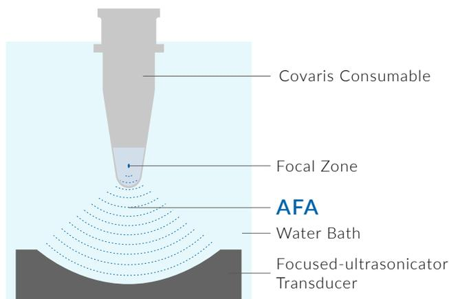
Adaptive Focused Acoustics (AFA) is an advanced acoustic technology which enables the mechanical processing of samples through focused-ultrasonication. AFA employs highly controlled bursts of focused high-frequency acoustic energy to efficiently and reproducibly process samples in a temperature-controlled and non-contact environment.
