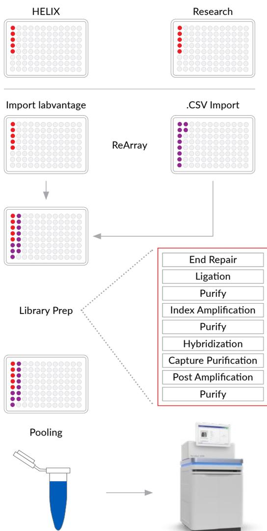
**Figure 1.** Experimental diagram of the library preparation workflow on the Hamilton STARplus. 32 samples are processed per run, with the ability to increase to 64 samples.
