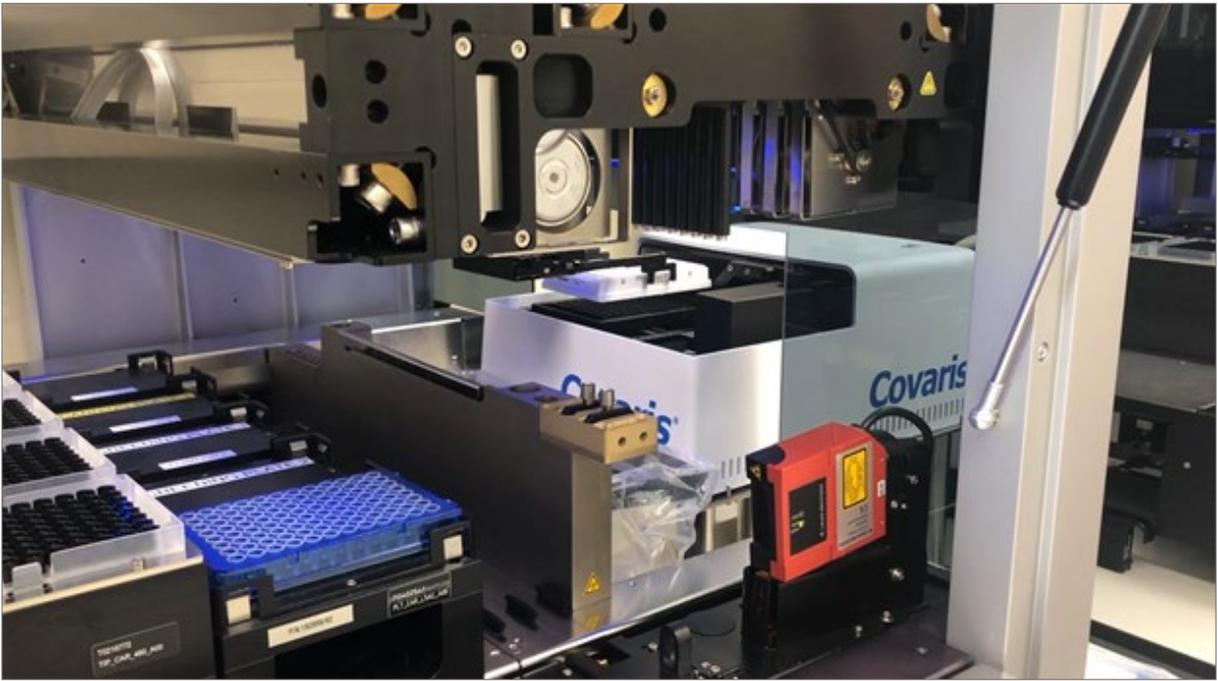
**Figure 3.** Picture of the R230 Focused-ultrasonicator integrated on deck with the Hamilton STARplus. This R230 is integrated onto the deck of the STARplus used for sample normalization
